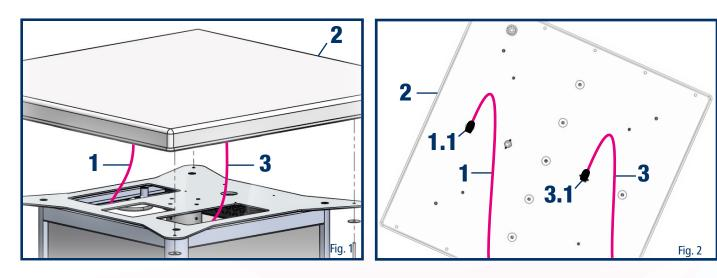
The following section explains how to route the cables for the twall® S (with light base). See Fig. 1 + Fig. 2.
