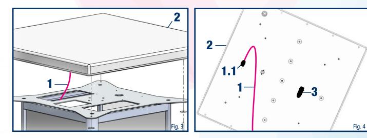
The following section explains how to route the cables for the twall® S (without light base). See Fig. 3 + Fig. 4.
