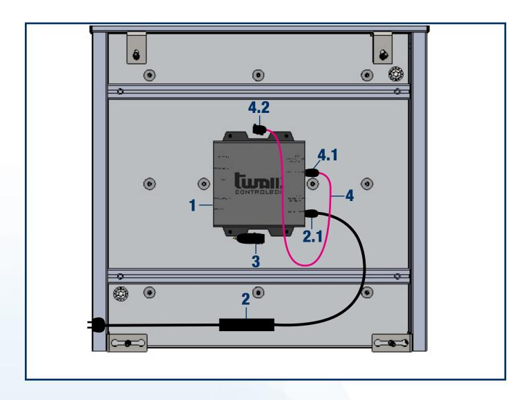
The following describes the installation of the connection lines for the **t**wall® D1 (solid variant).
